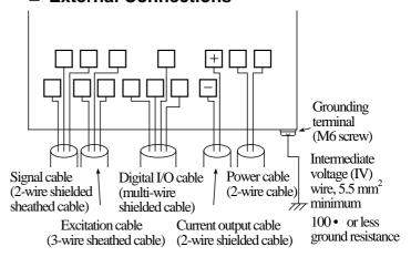
Figure 8. Converter Terminal Connections
